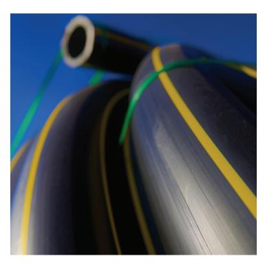
United Poly System D2513 HDPE pipe is used for pressure applications in the oil and gas industry. It is manufactured in IPS and DIPS (4 in. and up) sizes and meets or exceeds ASTM Standard D3350 requirements for polyethylene pressure pipe. The product is manufactured with a yellow print line for identification.
