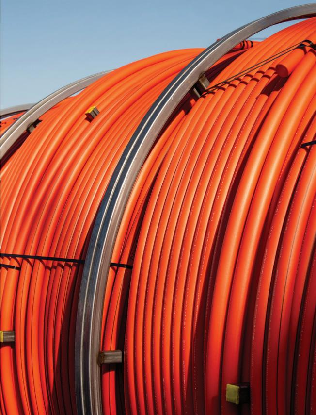
United Poly System's Comm-Line is one of the most common conduit solutions for telecommunications and fiber-optic projects across the United States. It is available in IPS (Iron Pipe Size) in diameters from  $\frac{3}{4}$  to 16 inches and DIPS (Ductile Iron Pipe Size) in diameters 4 inches and up. It can be installed in existing conduit or via plow, direct burial or HDD (horizontal directional drilling) installation methods.
